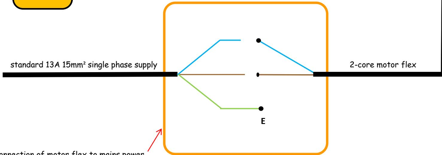
connection of motor flex to mains power (e.g. 'Klix' socket, spur unit, etc.)
