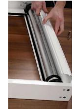
Remove the cover plate screw and carefully take off the cover plate.
