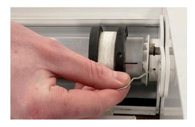
Press and hold the reset button (using a pin) till the blind shunts (moves) a couple of times. The motor is now activated and the blind is ready for pairing.
