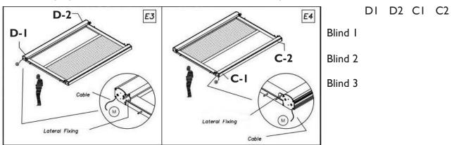
PLEASE NOTE: THE SKYFIT MOTORISED BLIND HAS THE **MOTOR IN THE FOOT OF THE BLIND** (THE OPPOSITE END TO WHERE THE FABRIC COMES OUT OF)
